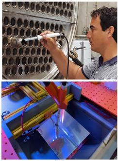
• In one step, this method cleans, passivates and polishes metal surfaces electrochemically. Polishing drastically reduces the incrustation of subsequent contamination, an added bonus of this specific method. The switchable AC/DC devices also facilitate direct current (DC) mode for high-gloss polishing.
